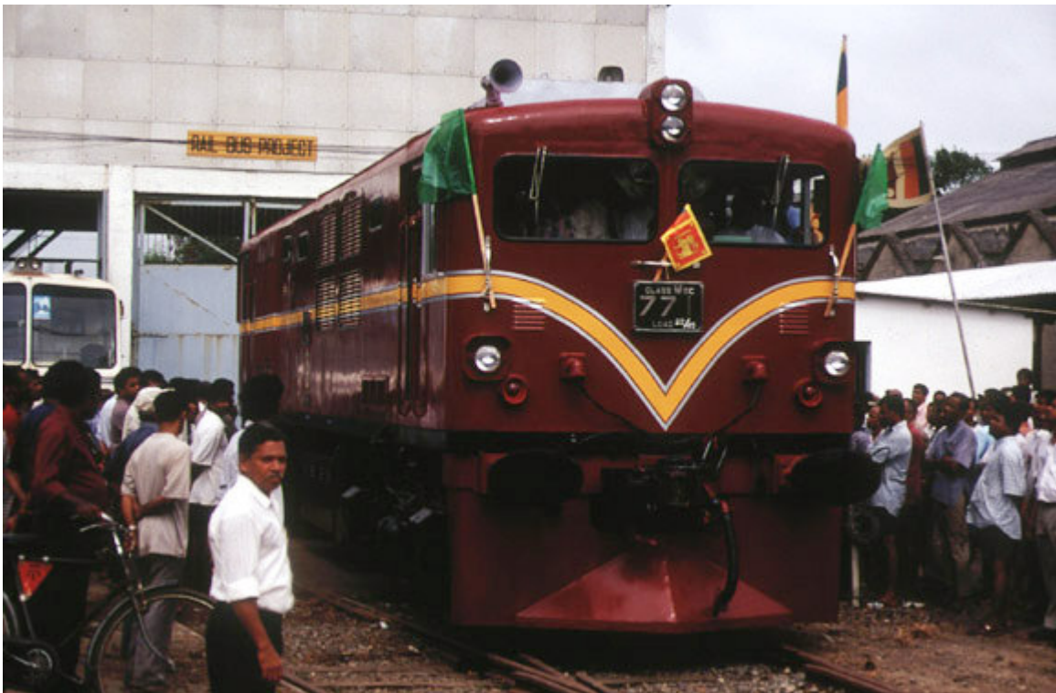
M5 C AT RATMALANA Four M5s have been rehabilitated with Caterpillar engines. The last of these, No. 771, was commissioned on 16 July 2002 and immediately hauled a special train from Ratmalana Works to Fort. [DH, 16 Jul 2002]
