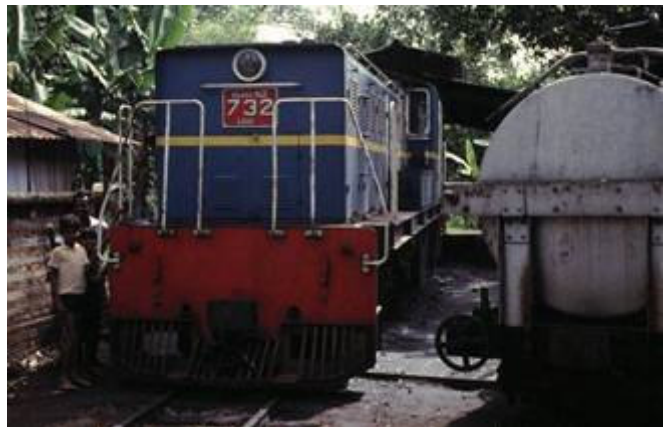
AVISSAWELLA SHED with Class N2 locomotive number 732 waiting overnight to head the morning train to Colombo. Note the narrow gauge oil tank wagon for refuelling locomotives at Avissawella. [DH, 19 Aug 1990]
