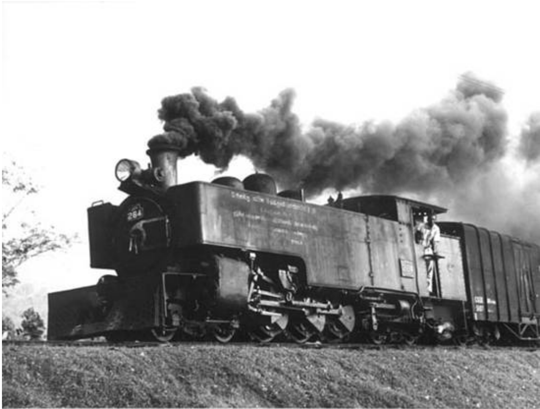
OIL-FIRED J1 A NEAR KURUWITA Both these photographs show No. 264 hauling freight trains near Kuruwita. In the photograph above, taken in 1973, No. 264 had just been converted to oil firing and carries a Sinhalese inscription which translates as: According to a recommendation by employees of the locomotive division [abbreviations of a division], converted to oil by railway employees at Dematagoda Workshop No. 1. [LAN, Nov 1973 and Mar 1974]
