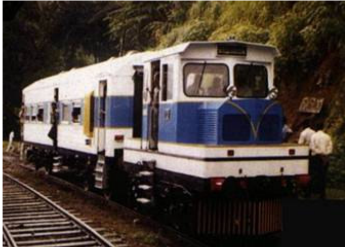
LEFT: MINI-LOCO ML1 The present GM(T) and former CME, Mr P.P. Wijesekera, has for some time pursued the use of cheap, easily available bus engines as an alternative to conventional railway motive power. Mini-loco ML1 was an attempt to produce a low-cost locomotive suitable for hauling one or two coaches on Up Country gradients. It was built in 1999 as a prototype for an intended 30 locomotives of this type. Direct interest in this project has now waned and has been transferred to producing a number of fibre-glass-bodied 3-coach sets powered by two bus engines. This picture of ML1 was taken at Balana, probably in 1999 [SLR]
