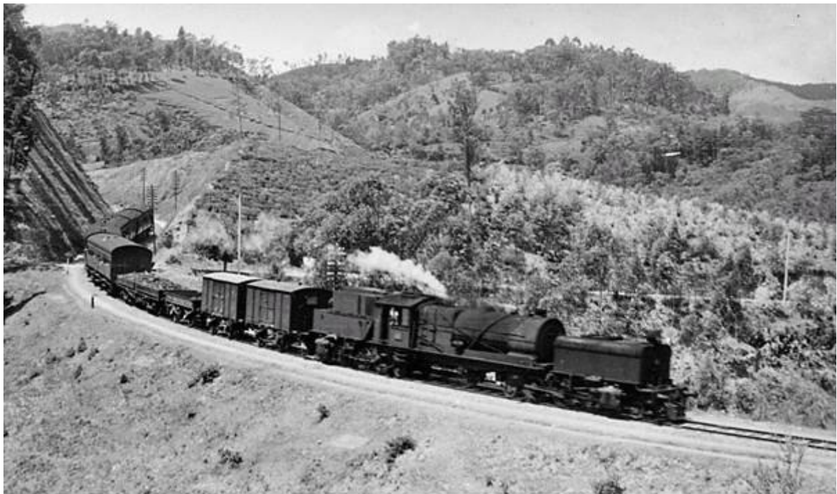
TWO PICTURES FROM THE 1940s or 1950s Mr David Ruston sent me five scans of pictures taken by his father, the late Mr T.A.M. Ruston, Locomotive Foreman at Ratmalana in the 1940s and 1950s, two of which are shown here. Above, an unidentified Bayer-Garratt (C1A) is hauling a mixed train possibly just beyond Hatton and, on the next page, B2 A number 3 is halted at a water tower but the location is not known. [T.A.M. Ruston, date unknown]
