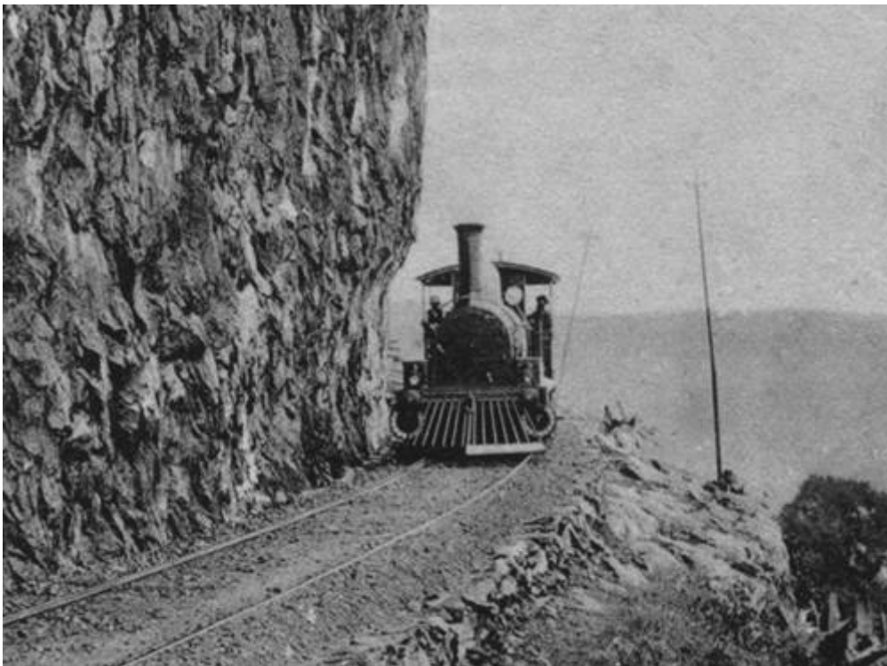
EARLY LOCOMOTIVE ON THE KADUGANNAWA INCLINE This must be one of the Fowler 0-6-0 tender freight engines of Class F as these had outside cylinders but it seems small and primitive for one of these. However the only other outside-cylinder engines in the early days were the Stephenson 0-4-0ST shunting engines but they were saddle tanks! [Restored by DH from a photograph in the Frederick Mendis Collection]
