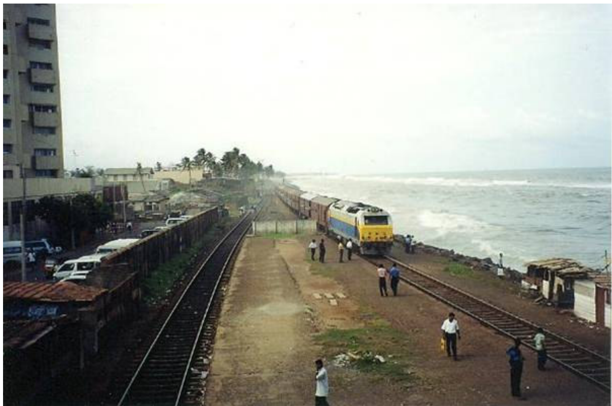
RUHUNU KUMARI AT BAMBALAPITIYA This relatively recent picture of an Alstom M9 locomotive heading up Ruhunu Kumari through Bambalapitiya makes a very interesting comparison with that classic picture of an M1 doing the same thing in 1964 (plate 20A in RSL ). Note the mist from the sea spray which accounts for the heavy corrosion experienced by both track and trains on the Coast Line. [George Pereira, 25 Oct 2003]
