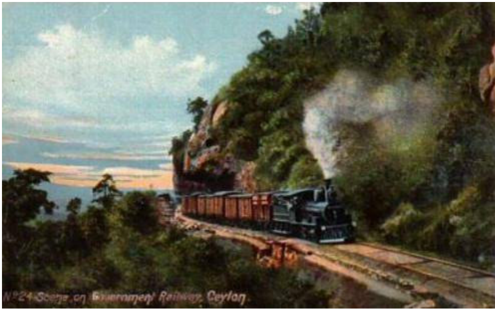
FREIGHT TRAIN AT LION ROCK ON THE KADUGANNAWA INCLINE A scan of an old postcard. The locomotive appears to be a Fowler Class F 0-6-0 freight locomotive (c.f. Plate 42 in RSL ). As these locomotives were withdrawn in 1912 and 1914, this picture must date from the early 20th Century at the latest.
